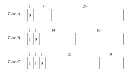
■ for example 193.63.129.1 is a class C address as we convert the first byte of the address 193 into binary and examine the top 3 bits of a byte
